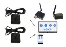
2. Use iGS01S or iGS02E beacon gateway to receive the beacon message and send to cloud server. User can access and manage the data anytime anywhere.
